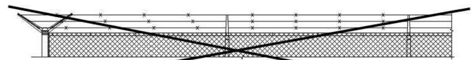
TYPICAL 6 STRAND BARBED WIRE AND DOUBLE EXTENSION ARM CONFIGURATION
