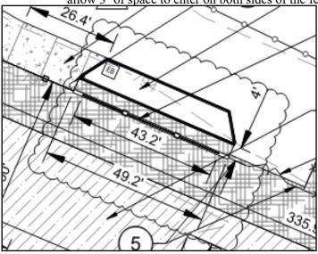
2. C201 – Dimensions for proposed warning track has been added to improve clarity
