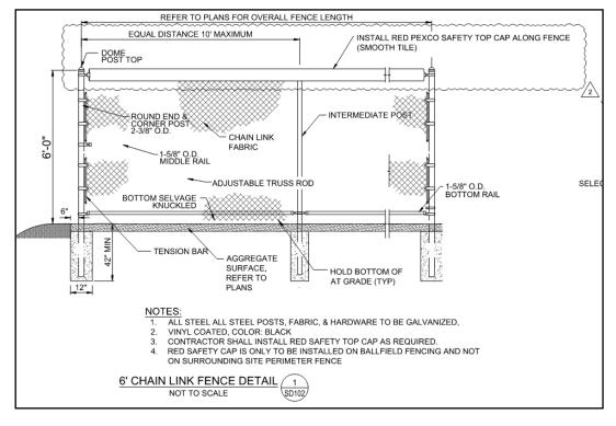
5. SD102 – Detail 6 on sheet SD102 has been updated to show the direct embed foundation as mentioned in Part 4.
