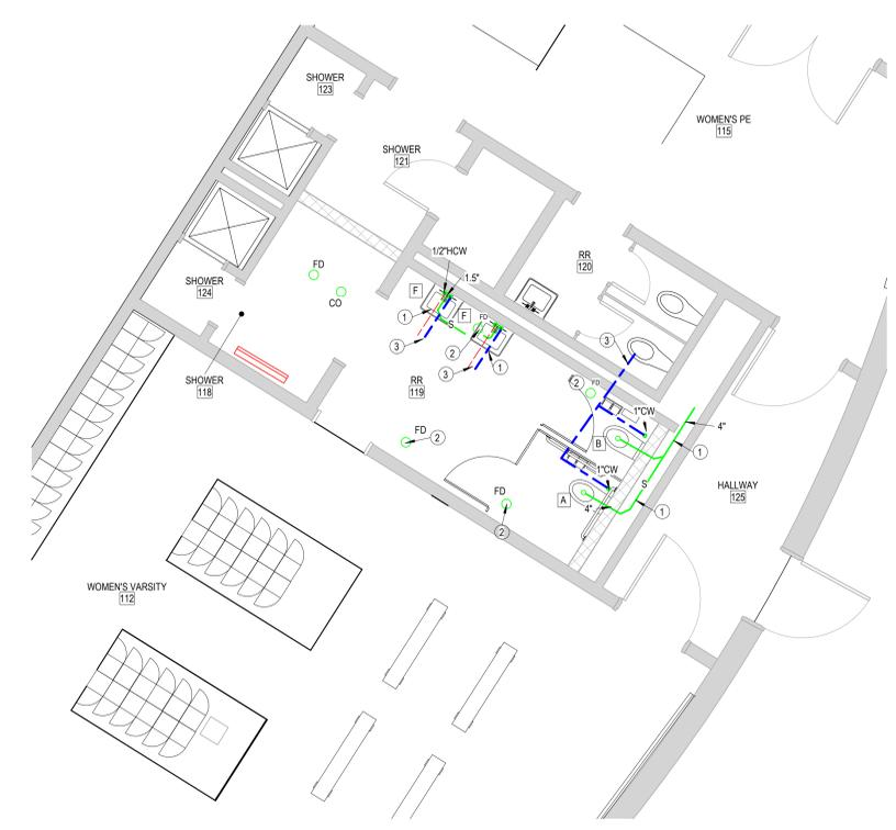
1 LOWER LEVEL PLUMBING FLOOR PLAN
