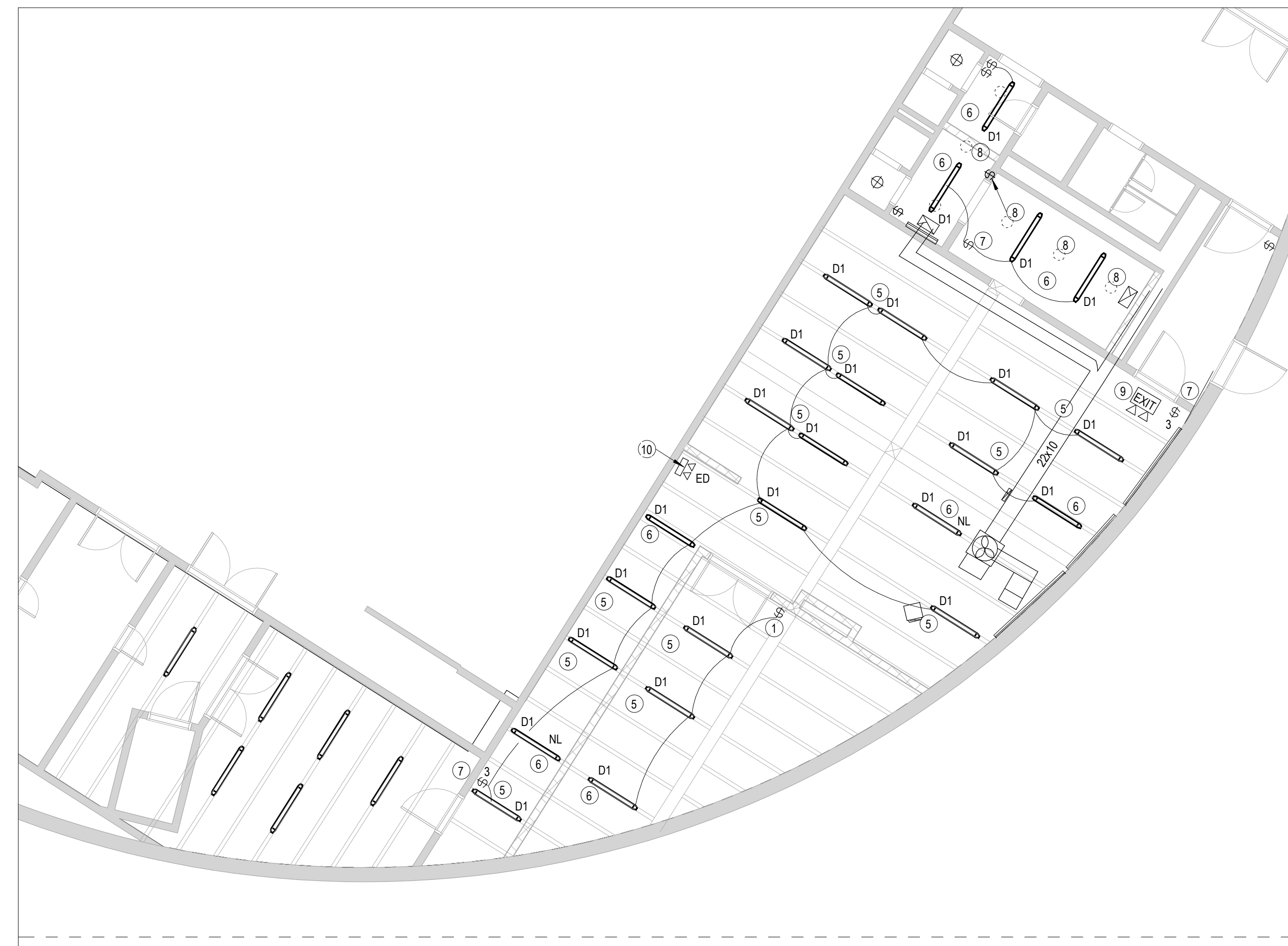
8 LOWER LEVEL ELECTRICAL LIGHTING PLAN SCALE: 1/8" = 1'-0"
